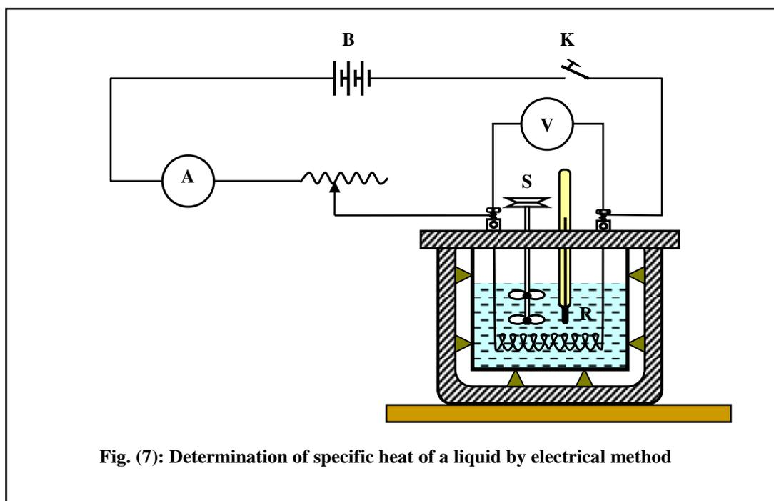
The liquid, whose specific heat is to be determined, is poured into the calorimeter until the coil is completely immersed in it. The mass  $m$  of the liquid taken is known by weighting the calorimeter first empty and then with the liquid.
