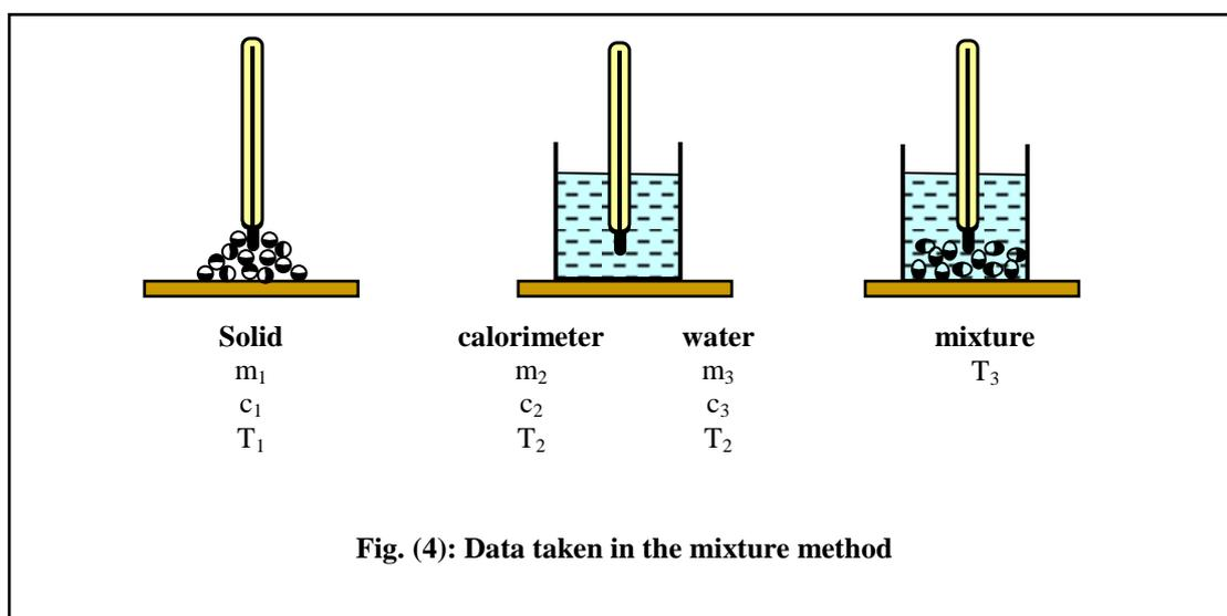
Suppose  $c_1$  is the specific heat of a given solid.  $m_1$  grams of the solid at  $T_1$  °C is added to  $m_3$  of water at  $T_2$  °C in a calorimeter whose mass is  $m_2$  and its specific heat is  $c_2$ . Let  $T_3$  °C be the final temperature of the mixture, see Fig. (4). By equating the heat lost by the solid  $Q_s$  to the heat gained by the calorimeter and water ( $Q_c + Q_w$ ) we get
