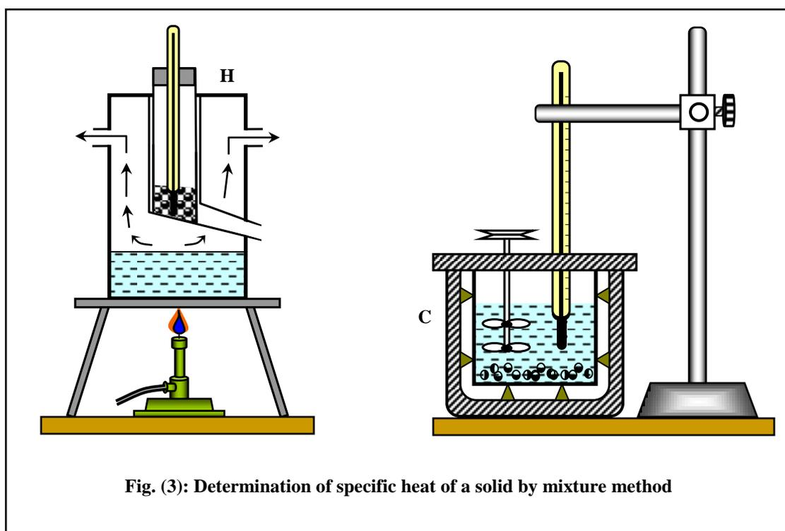
The solid, in the form of a small pieces, is weighted and suspended inside the heater by a thread passing through the cork. Steam is passed
